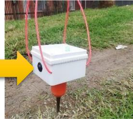
Nail the module firmly in the ground and turn it on through the side switch, (the top led will light up).
