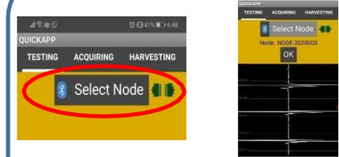
In the Testing tab select the node and then press TEST. To see the signal in real time. (do this for all nodes)
