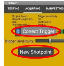
Locate the trigger node at the chosen point, select connect trigger and then new trigger point.
