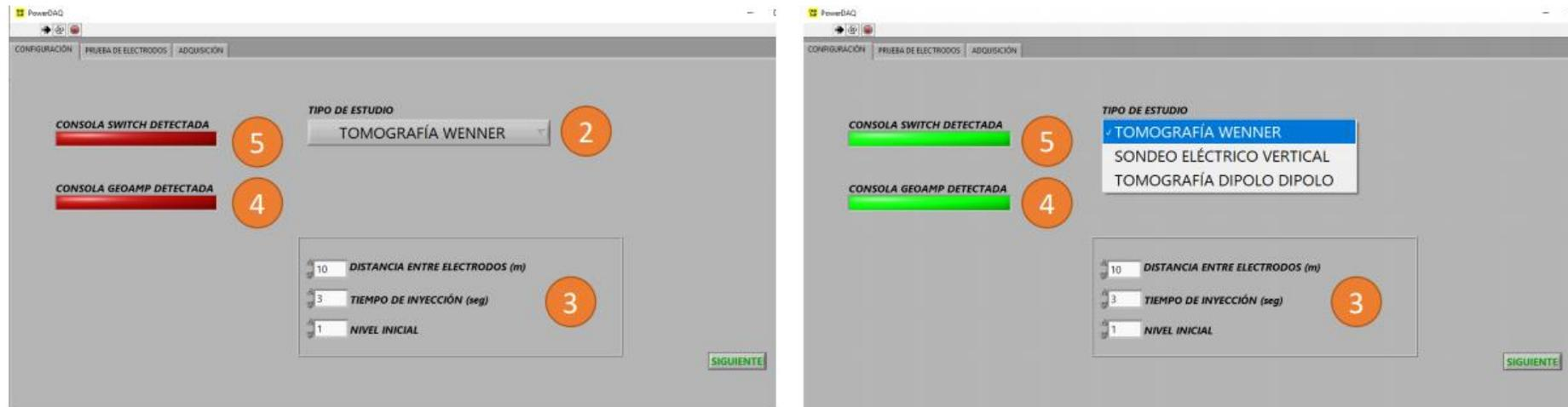
\* You will not be able to go to the acquisition tab ("NEXT" button) if any of the consoles is disconnected.
